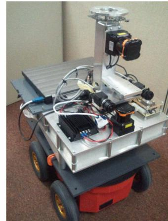
Fig. 1. The Pioneer platform with the computing laptop and the scanning lasers. The coronally-scanning Hokuyo laser is mounted on the sensor mast, while the horizontally scanning unit is mounted at the front of the platform.
