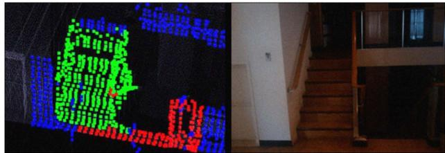
Fig. 7. Example of detection of a door and a staircase. Red points mark the two sides of the detected door and green points mark the staircase. Unlabeled points are colored blue. The image is shown only for reference.
