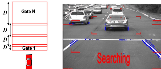
Figure 1. Detection gates. Left: An overhead view showing a set of N gates ahead of the vehicle, each of which covers an equal number D stereo disparities. Right: Red reticles show the detection gates projected onto the image plane. Blue pixels show ground plane points.
